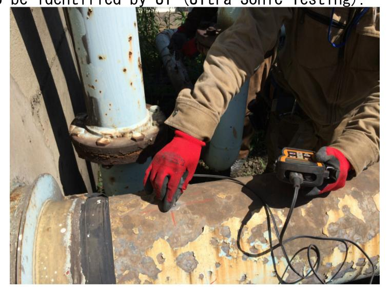
The pipe thickness measurement using UT is to make a double check on our EPD measuring data, which is to follow Japanese Industroial Standard (JIS Z 2355) requirement.
