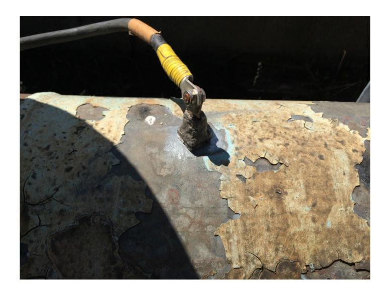
The same to fix the electrode(s) by magnets.
