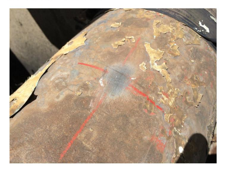
To polish the surface until it appears the original steel color. The area for sensor pin needs to be 20mm\*20mm, the area for electrode needs to be 40mm\*40mm around.
