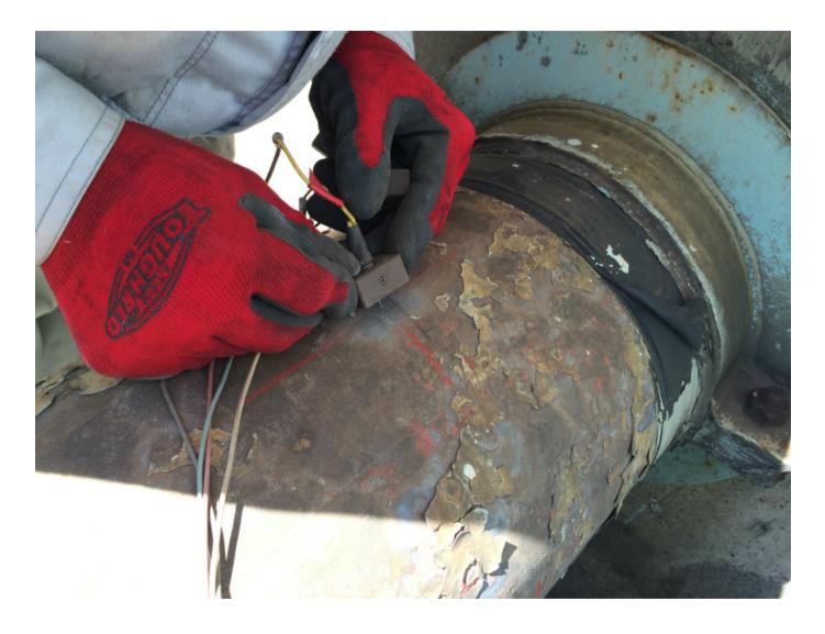
The sensor pin having a built-in magnet can be easily fixed on the pipe. In case of a stainless pipe, the sensor pin having a dual side sticker can be fixed on the pipe.
