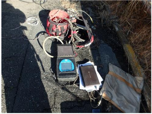
Hardware and program set up, voltage difference measurement and data acquisition/confirmation are all managed via laptop and EPD device.
